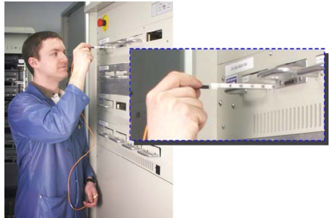
Figure 2: The spectral probe enters a vertical slot next to each fixture on the front panel of the LRS-9550 system. Numbered lines on the probe indicate which device the probe is measuring.
