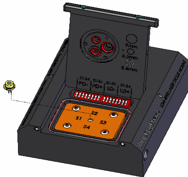
Figure 2.7 Installation of a 9.0 mm Window Can Laser
